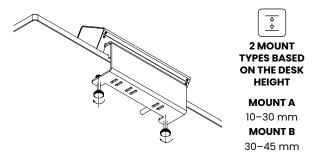
No tools are needed for this installation. You need to choose size of the side mount before you order the panel (10-30 mm or 30-45 mm).
