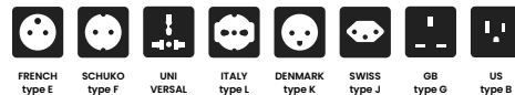
FRENCH type E SCHUKO type F UNI VERSAL ITALY type L DENMARK type K SWISS type J GB type G US type B
