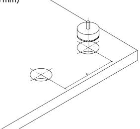
**3|**Take a jig saw and cut the space between the holes
