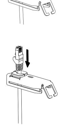
3 | Clip the plastic fastener on the cable to the metal head
